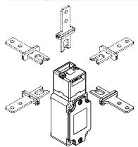
Removing the two fastening screws, in all switches, the head can be rotated in 90°
