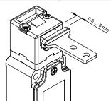
This switch has a wide backlash of the actuator into the head (4,5 mm) for an easier installation. With closed door, check that the actuator doesn't knock straight against the head of the switch; it must be in the adjustment zone (0,5...5 mm)
